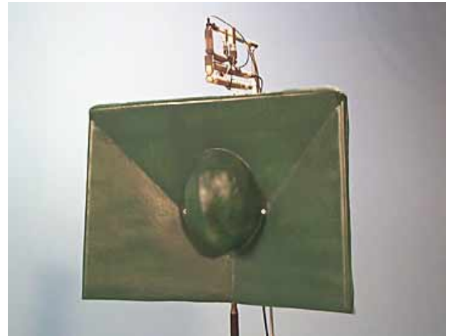
Fig.4 - PerAmbio 3D/2D microphone array combines a baffled pinna-less ellipsoid “Ambiophone” developed by the author and a 1 st -order (B-format) Ambisonics microphone atop realized using high quality discrete capsules. Note that the transducers of the Ambiophone are at human ear positions.
